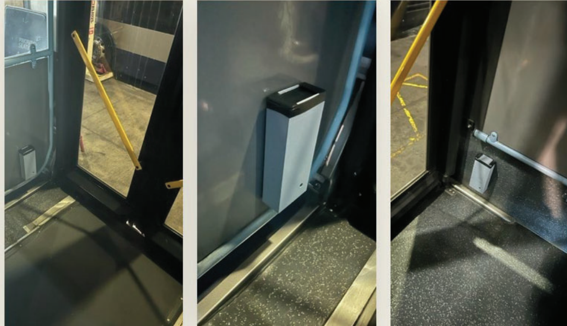
Figure 6 – On-to-Off Recording Device and Positioning
